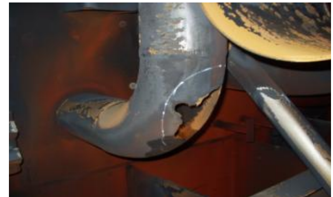
Changing steam conditions cause FAC in heaters, extractions, drains
