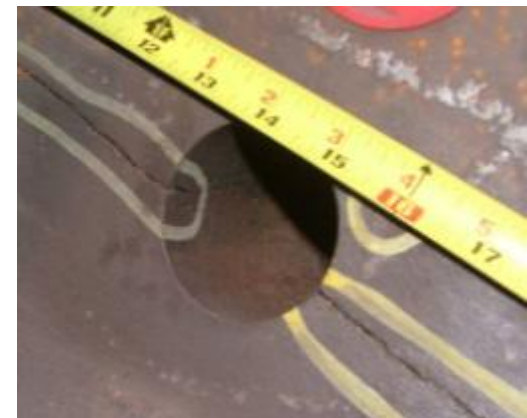
Ligament cracking in boiler header
