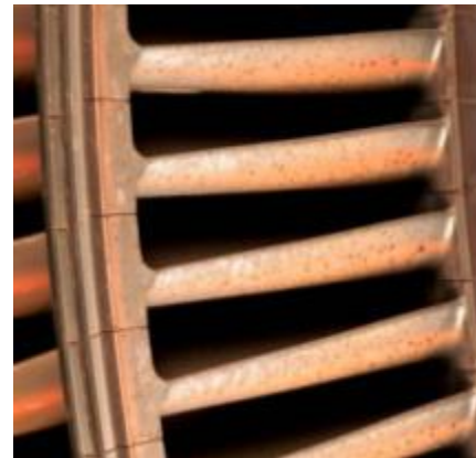
Pitting on steam turbine rotor
