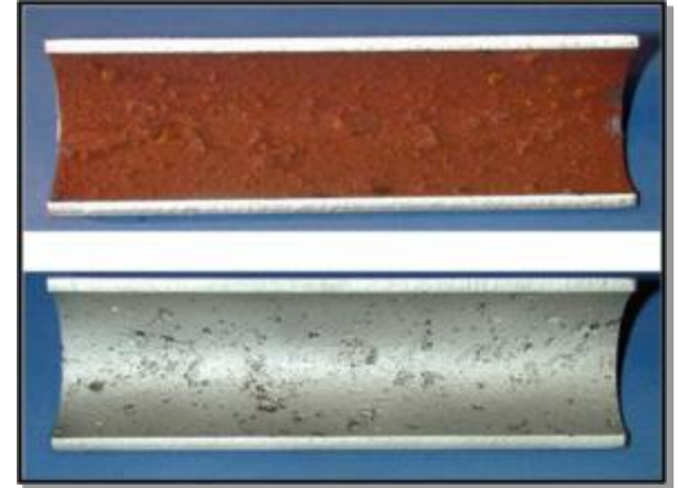
Corrosion in boiler tubes
